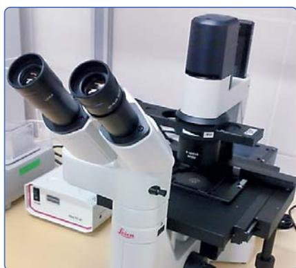
Inverted microscope with fluorescence module
