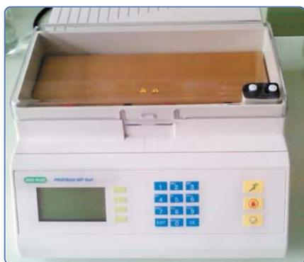
Apparatus for isoelectric focusing
