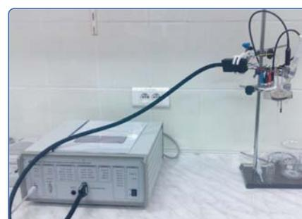
Potentiostat for anodic stripping voltammetry (ASV)
