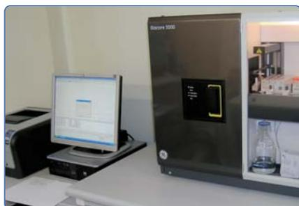
An instrument for real-time analysis of macromolecular interactions
