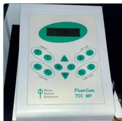
Flurometer for measurements of in vivo chlorophyll fluorescence equipped with a FluorCam 701 MF imaging unit
