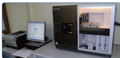
Instrument for real-time analysis of macromolecular interactions
